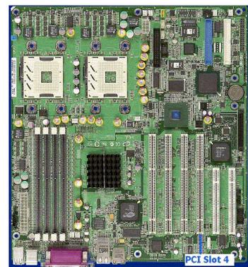
Gráfica 52. Tarjeta madre con Ranura PCI. Fuente: [http://www.intel.com/support/pix/motherboards/server/pci\\_slot.gif](http://www.intel.com/support/pix/motherboards/server/pci_slot.gif)
