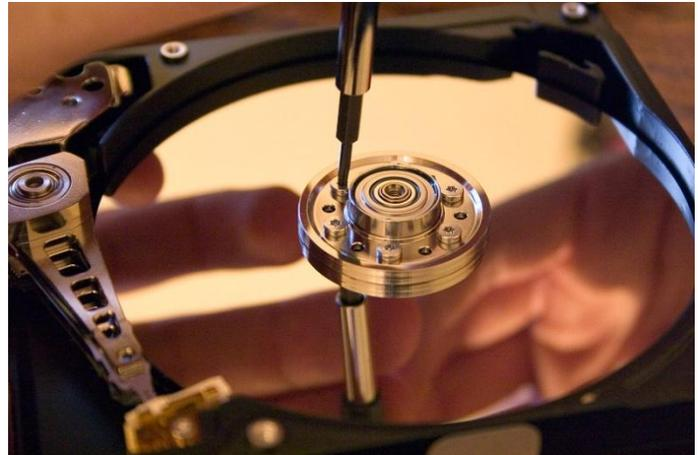
Gráfica 42. Disco Duro interno. Fuente: [http://upload.wikimedia.org/wikipedia/commons/1/1d/Hard\\_disk\\_platter\\_reflection.jpg](http://upload.wikimedia.org/wikipedia/commons/1/1d/Hard_disk_platter_reflection.jpg)
