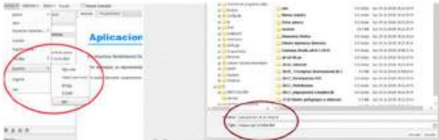
Figure 5. The eXe learning integrated material is exported as a IMS zip file to the Moodle platform
