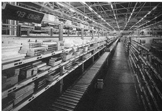
(Figura 7.18) Paper-less, picking to light
